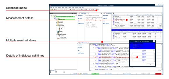
Image: Display of the results from a runtime measurement using CODESYS Profiler
